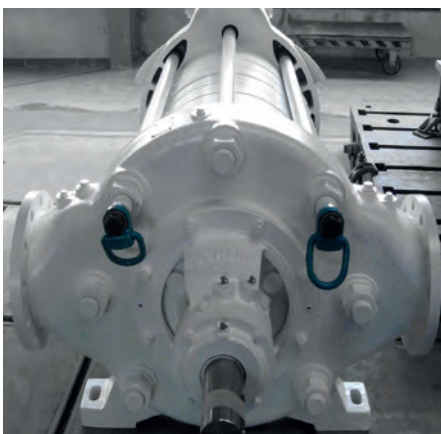
Two flanges in one suction casing
